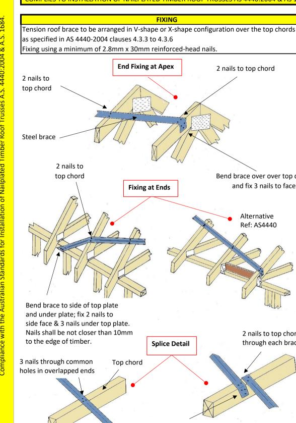
Bend both ends of brace over chord; fix with 3 nails each side
